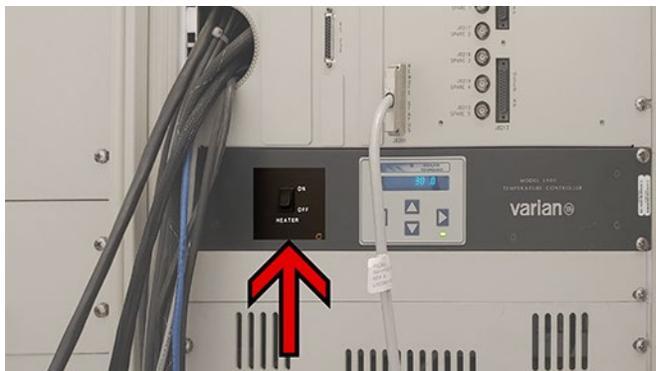
8. Wait at least 10 minutes once the instrument reaches the set point for the temperature to equilibrate across your sample. If changing the temperature by 10°C or more, or running quantitative NMR, you should tune the probe.
